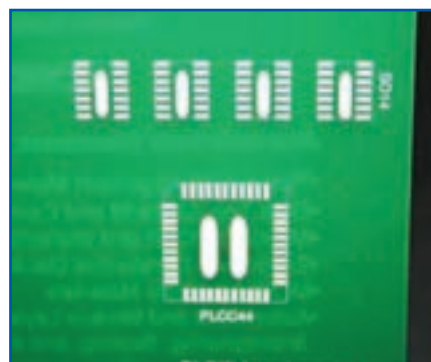
Figure 5. Demonstration of stencil printability of A-1 onto FR4 board.
