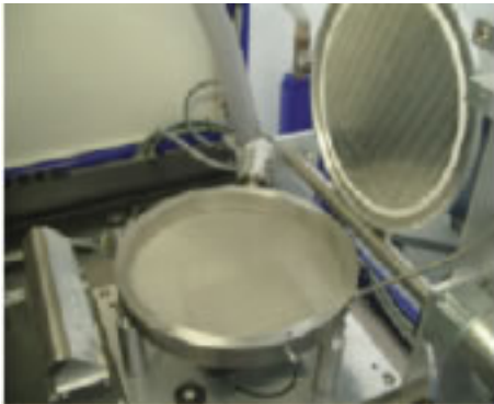
Figure 2. Solder sphere reservoir filled with solder spheres.
